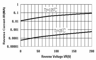
Fig.2-Typical Values Of Reverse Current Vs.Reverse Voltage
