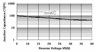
Fig.3-Typical Junction Capacitance Vs.Reverse Voltage
