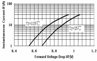
Fig.1-Typical Forward Voltage Drop Characteristics
